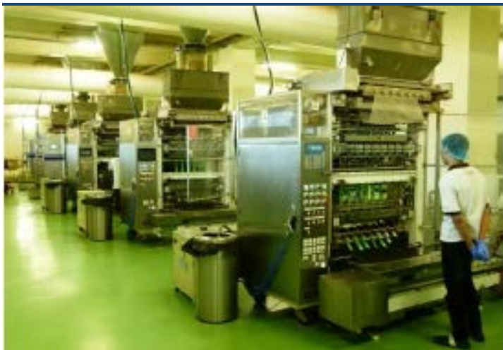
Figure 6 : Automated 6-lane packaging machines
